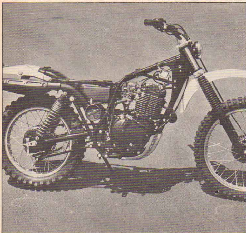
DR frame and swing arm are strong, flex-free items. Rear brake is full floating but still chatters if used hard.
