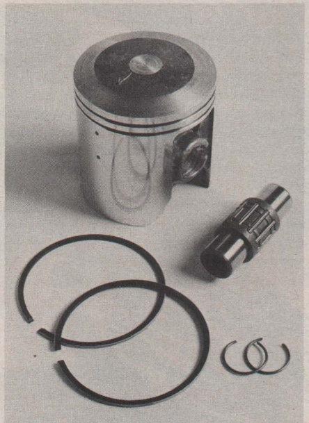
Rectangular-section rings limit blow-by, while piston skirt holes allow oil up to the bridge on the exhaust port.
