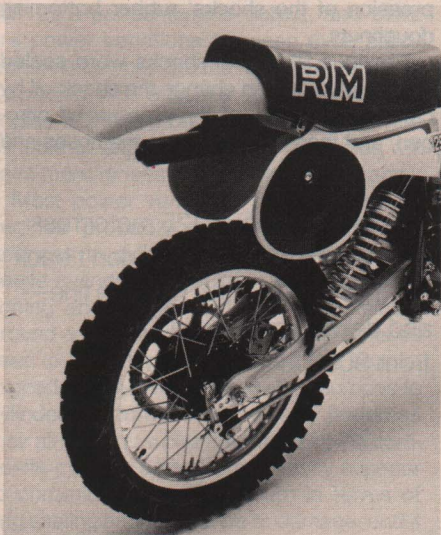
A naked brake-actuating cable replaces last year's rod, though the cable transmits less braking information.
