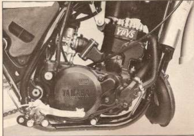
The latest YZ250 motor is liquid-cooled and Power-Valved Yamaha uses every trick in the updated motocross book.
