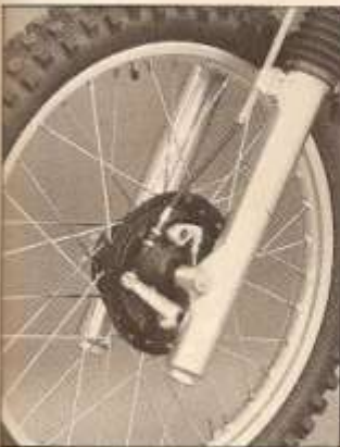
Kayaba fork has three adjustments
