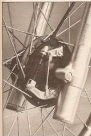
Double-leading-shoe front brake Shorter stops for the YZ250.
