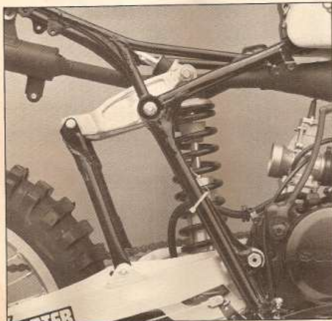
Aluminum is used to craft the Kayaba shock, bell crank and swingarm
