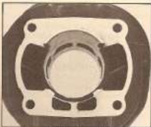
Booster exhausts above the transfers
