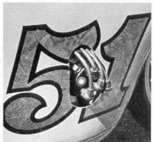
In order to use the distributor, it was necessary to cut a hole in the fairing to provide clearance.
