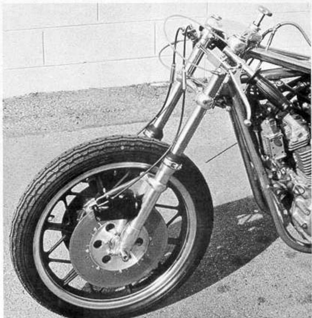
Standard road racing Ceriani forks replaced the stock BSA items. No more wiggles at the top end.
