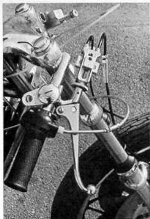
The original mechanical dual cable hook-up proved to be troublesome and ineffective.
