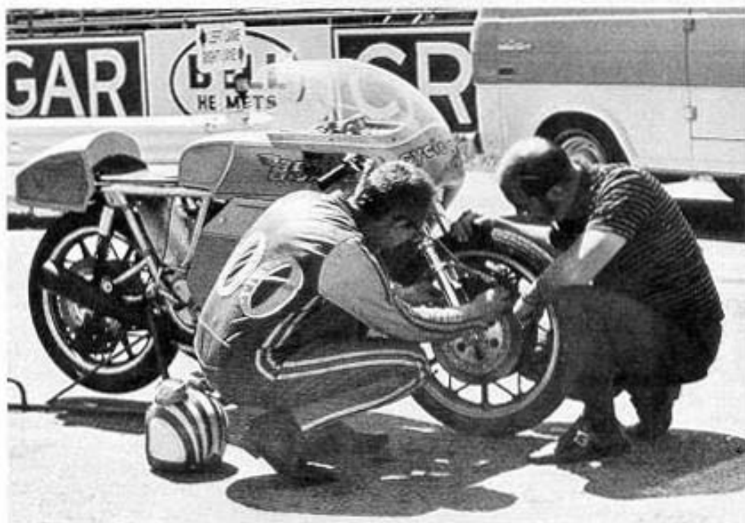
After repeated hard running, the discs turned blue (all three), but they didn't warp and the brakes worked fine.
