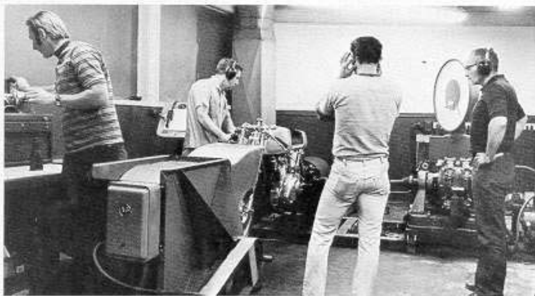
Dyno testing our jewel at Axtel's repeatedly produced astounding readings of over 70 H.P. at 7750 RPM.
