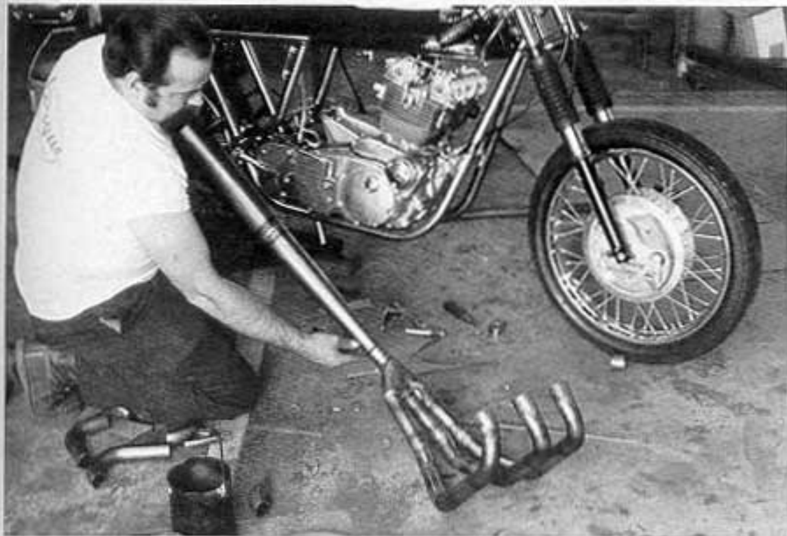
... he built this long, long megaphone as per the factory exhaust system specs.
