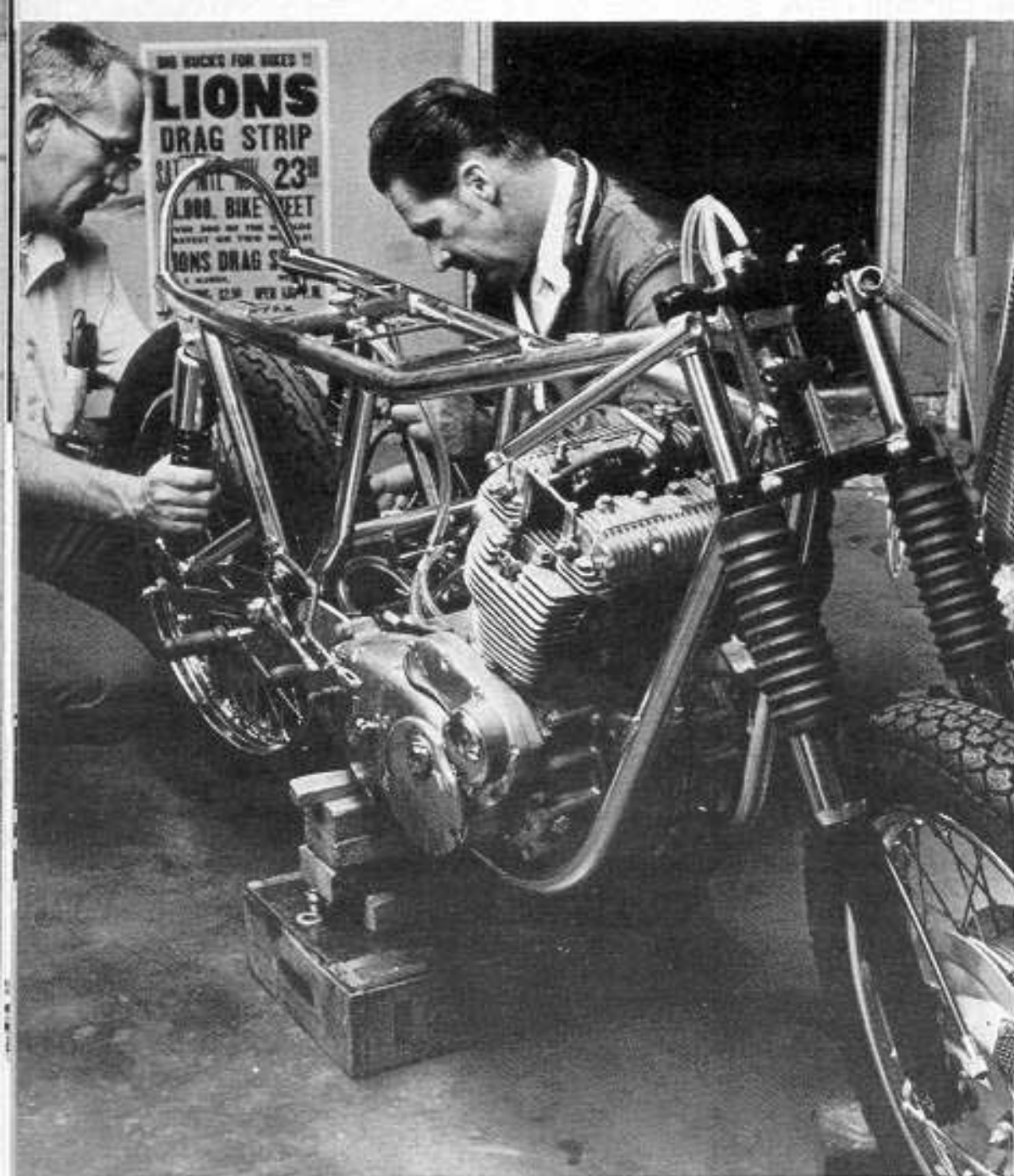
Jack Byers came over and gave me a hand on installing the rear wheel and had a few words of advice on the Rickman frame.
