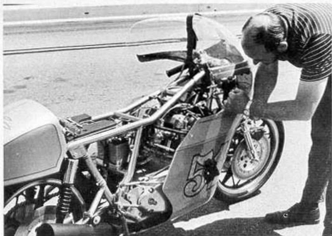
It took some additional jet work to get the engine sorted out the first time we went out to Orange County raceway.
