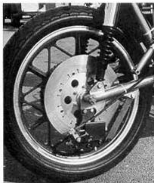
Once a heavier cable was used (it was necessary to use 1/8" cable), the single rear disc unit worked great.
