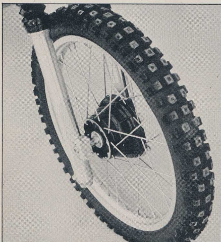
Front hub is a completely new design with straight-pull spokes. Brake backing plate is recessed and brake drum is placed closer to center of wheel, equalizing load on spokes. KYB forks have DU bushings for smoother action.
