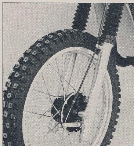
Front hub is a completely new design with straight-pull spokes. Brake backing plate is recessed and brake drum is placed closer to center of wheel, equalizing load on spokes. KYB forks have DU bushings for smoother action.
