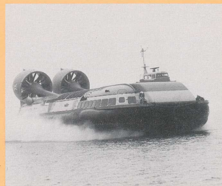
An early Vosper hovercraft equipped with Avon-designed skirt and fingers.
