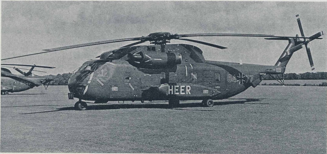
CH 53G SEA STALLION —A twin engine heavy assault transport helicopter that can carry up to 38 troops. Powered by two 2,850 SHP engines it has a maximum speed of 170 knots.
