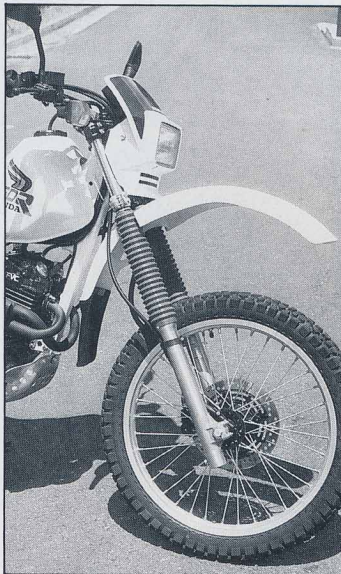
ABOVE The forks are way too soft for any serious dirt riding, especially in combination with the super strong front brake. On tar, the brake is excellent. We quite liked the Dunlop K550 tyre. Headlight is 12 volt with a quartz halogen beam, instruments are good, clutch is super light, controls are all comfortable.
