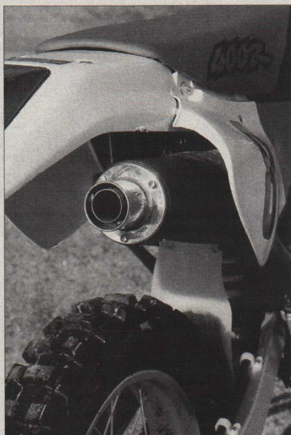
The '96 and '97 mufflers are the hot setup for the new XR. Swapping the end caps on the new model is worth 3hp, although the bike does get louder.
