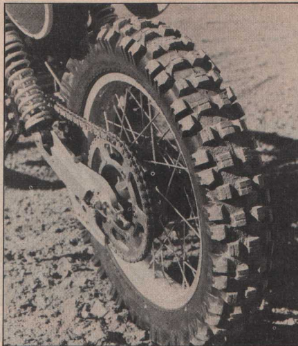
Our rear Dunlop worked well while the knobs stayed sharp, then deteriorated rapidly as they rounded off.
