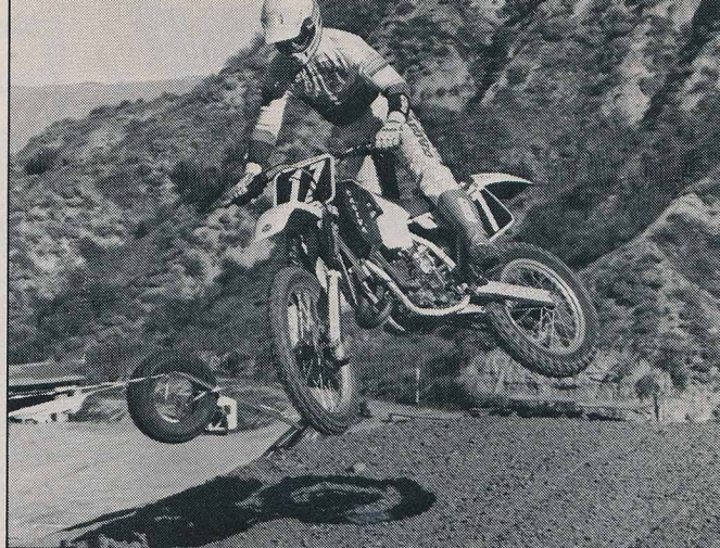
European: The Cagiva WMX 125's rapid-fire motor sits in a no-compromise chassis. A stiff frame/fork combination and smart geometry turns precisely and tracks straight.
