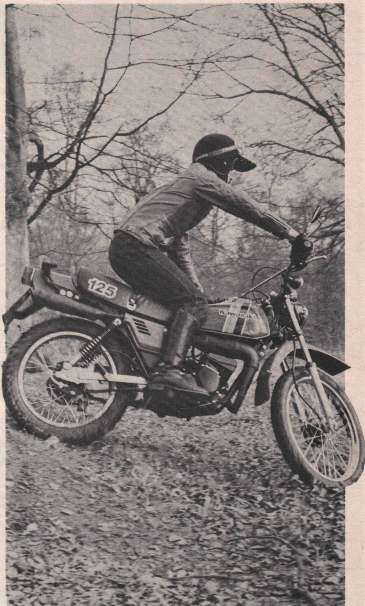
The Kawasaki KE125 is typical of the current range of Japanese two-stroke trail bikes - handy off-road and on.
