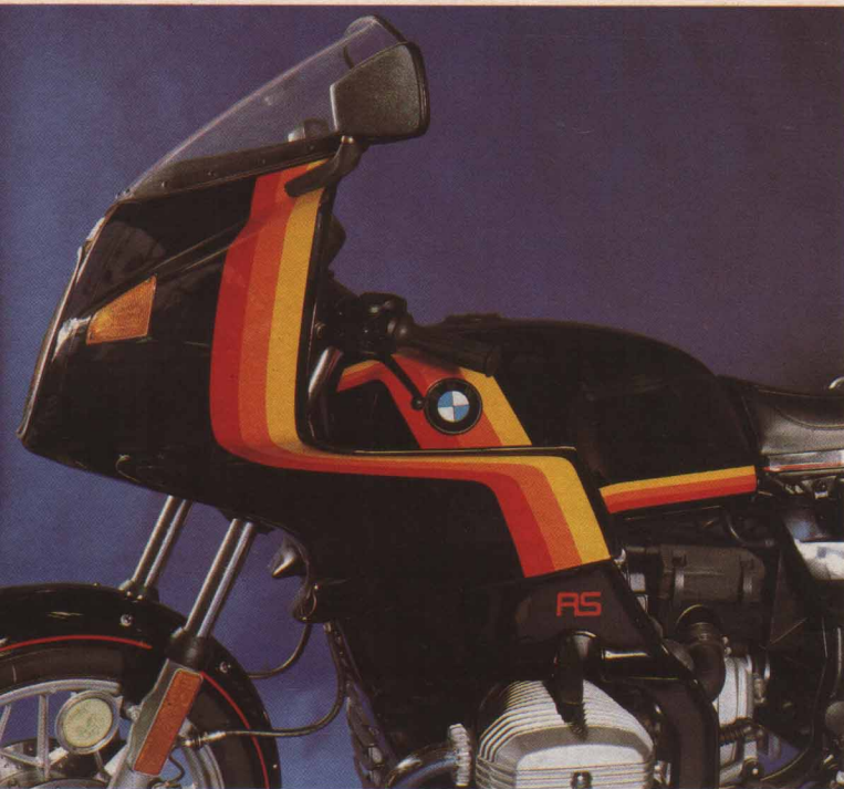
BMW R100 fitted with R100RS fairing and special paintwork.
