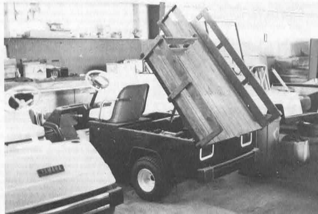
Yamaha Golf Car converted into a dump cart
