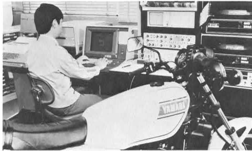
Computerized analysis of frame strength.
