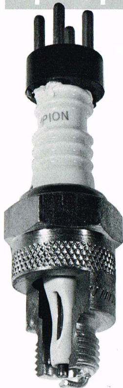
The sparkplug shown above is special. Its construction is identical to that of any normal type except in one detail. This plug contains a minute temperature sensing element called a thermocouple which is located at the tip of the insulator nose close to the centre electrode. These thermocouple plugs were developed by Champion Spark Plug Company to help them select the correct grade of plug for any engine.
