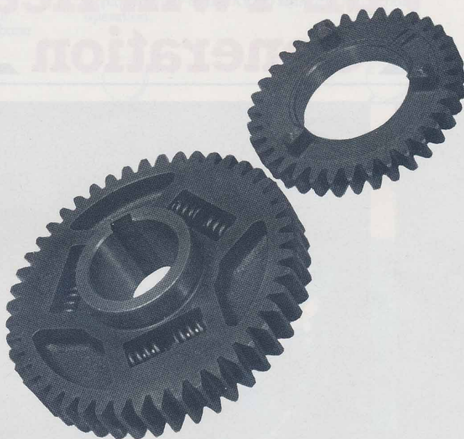
Side-by-side spring-loaded gears mesh with one another and are pre-loaded in opposite directions to maintain tension and so eliminate free play between the camshaft drive and idler gears. This cuts down both on wear and noisy "gear clatter" in the cam drive.
