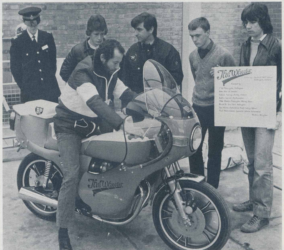
Gosford Hill School pupils designed "The Wheeler" and took second place. It has a novel fairing with twin windscreens for low and high speed riding, plus a number of anti-theft devices.
