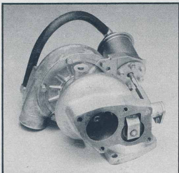
Borg-Warner mini turbo is 1/3 smaller than conventional units. The precision wastegate is built right into the unit and is fully adjustable.
