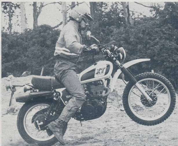
The XT500 is a little heavy for true enduro riding but makes a perfect dual-purpose machine. It has the performance necessary for street riding and its smooth four-stroke power makes it perfect for "green lane" going.
