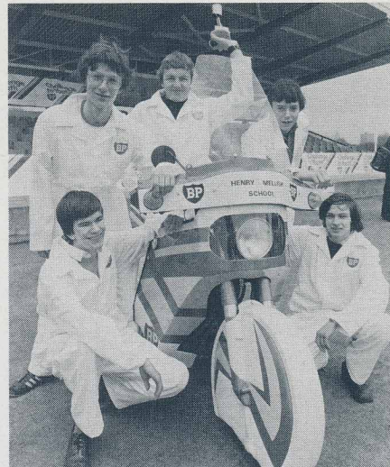
Enclosed front wheels and comprehensive streamlining aid in both weather protection and economy, thanks to better air protection, in the third place design of the Henry Mellish School.
