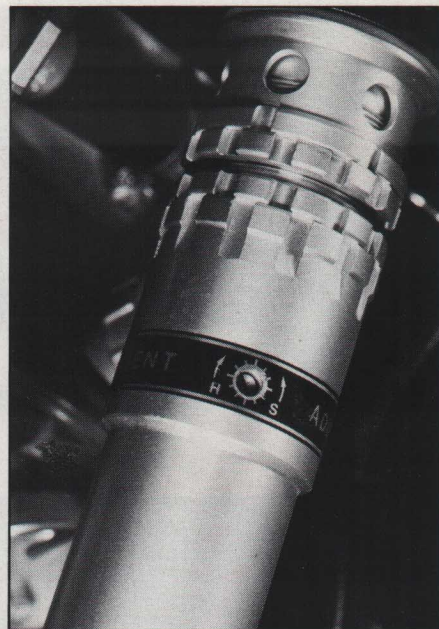
Left: A shot in the "heart" of the TZ250H. Separate cylinders and a new Monocross rear suspension are two of the most important modifications, compared with the previous TZ250 model.
