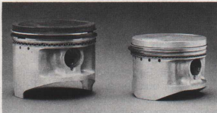
Clockwise from above: The 920 piston is a hefty 9mm larger in diameter. The two heads use the same castings, but the 920 has larger valves and a deeper combustion chamber. The transmission shafts are staggered vertically to reduce engine length. Screw-type valve adjusters make for easy maintenance by economy-minded home mechanics.
