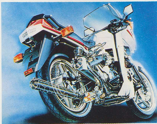
This drawing shows how the turbo-charger, driven by the exhaust gases, is mounted on the XJ650 Turbo.
