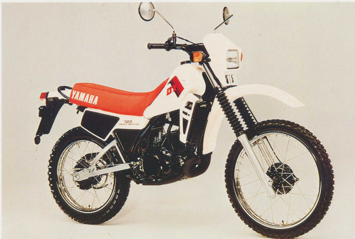
Moto cross inspired roadster – the DT125LC with water-cooled engine.
