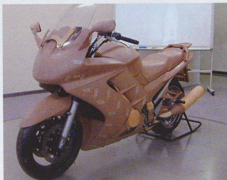
Clay model showing the unique design features
