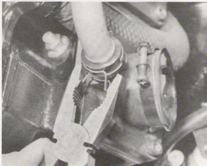
6.1b Note that pipe is held by spring clips which can be slid off after squeezing the 'ears' together as shown
