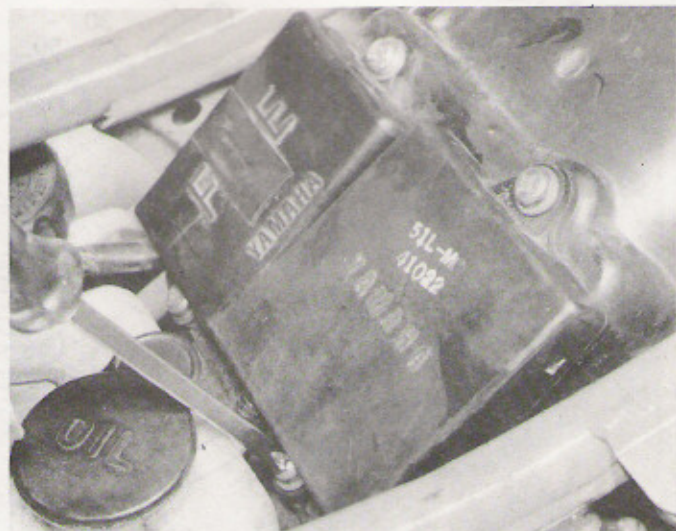
11.1b ... and remove YPVS control unit and fuse box from mudguard
