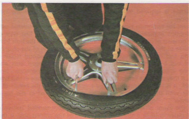
Use two levers to work bead over tyre rim
