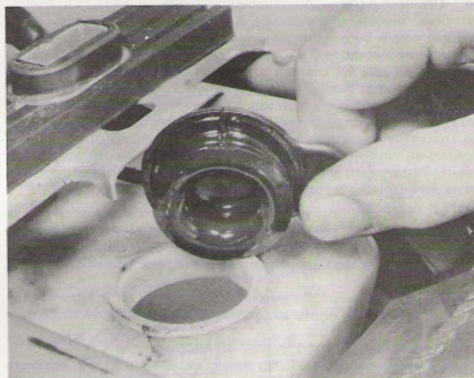
Engine oil tank filler can be reached after seat has been removed
