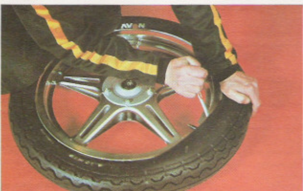
Use lever in final section
