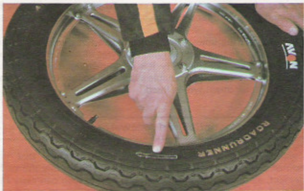
Tyre fitting: Replace first bead over rim noting arrow indicating correct direction of rotation
