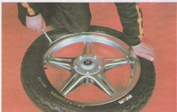
Work bead under rim towards and each side of valve using lever if necessary
