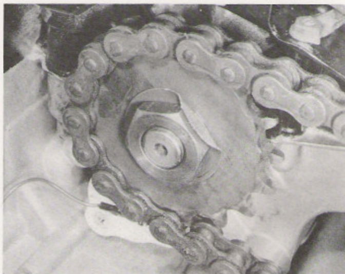
35.4c ... tighten securely and bend up the locking tab as shown
