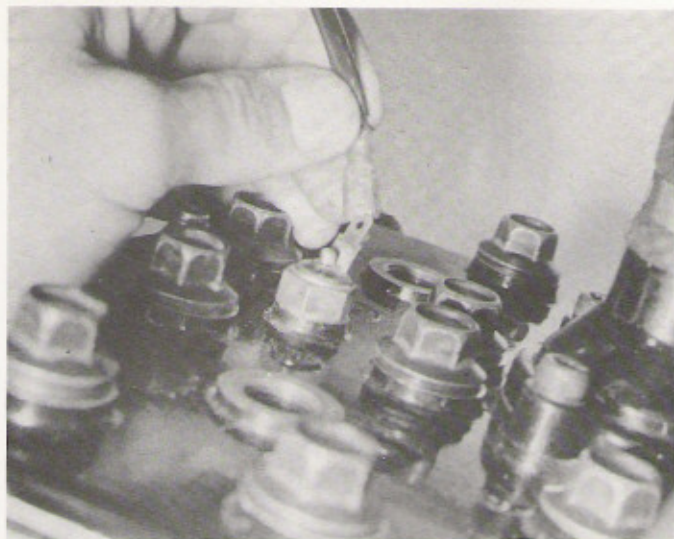
4.5b Disconnect the water temperature sender lead
