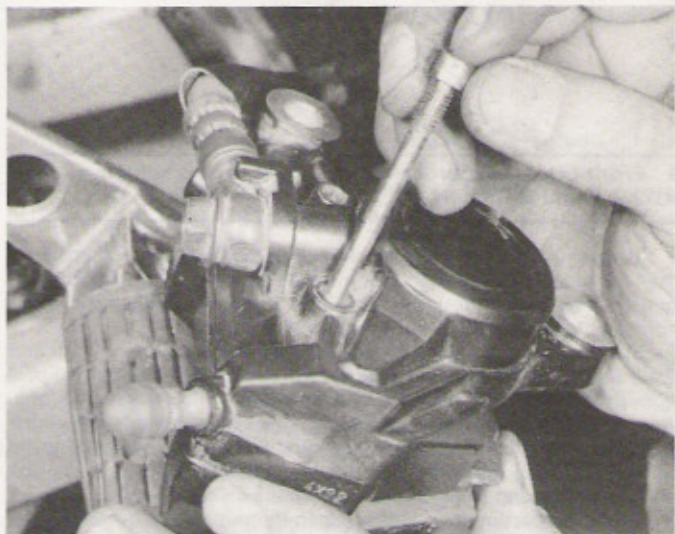
5.1d When refitting pads, hold them against the pad spring while the pins are inserted
