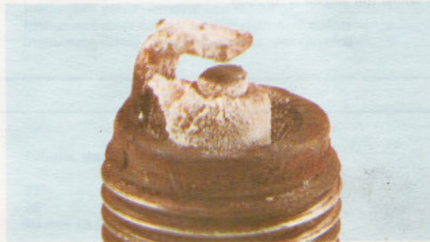
White deposits have accumulated from excessive amounts of oil in the combustion chamber or through the use of low quality oil. Remove deposits or a hot spot may form
