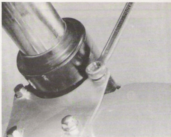
3.2b Remove outer bolts only to free mudguard and fork brace from fork legs
