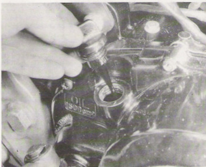
Transmission oil filler plug incorporates a dipstick. Level is measured with the plug resting on its threads – not screwed home
