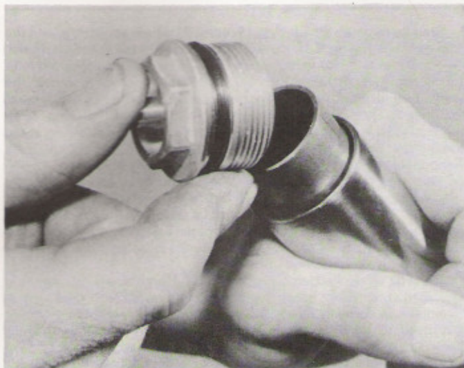
5.1a Remove fork top bolt ...
