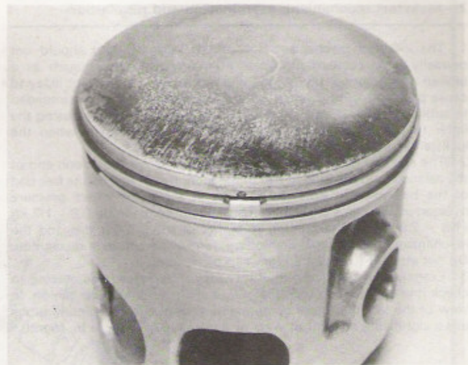
18.5a Note how ring ends locate over peg in ring grooves
