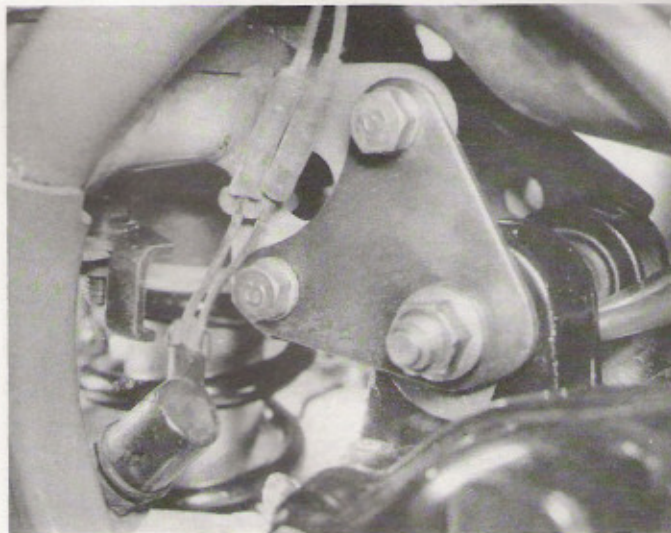
4.11b Upper rear engine mounting bracket arrangement
