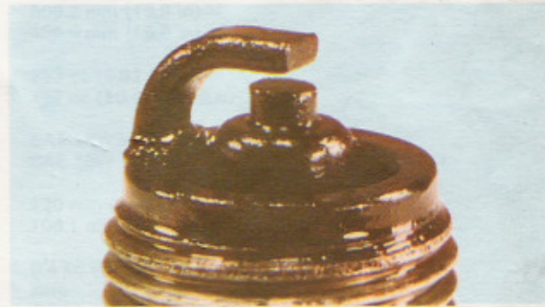
Wet, oily carbon deposits form an electrical leakage path along the insulator nose, resulting in a misfire. The cause may be a badly worn engine or a malfunctioning ignition system
