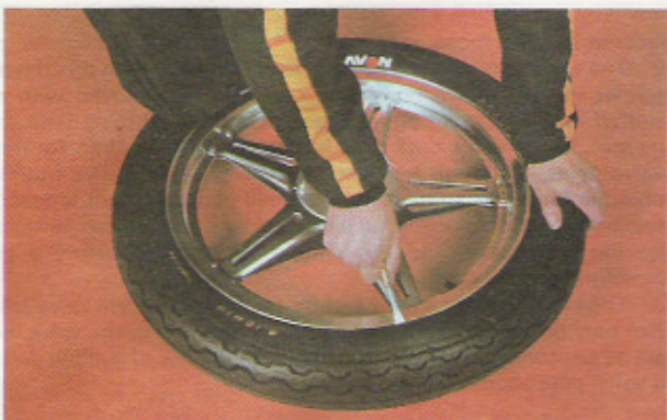
Tyre removal: Deflate tyre and insert lever in close proximity to tyre valve
