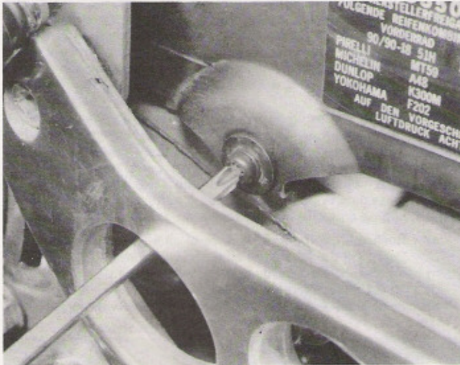
11.1e Chainguard is retained by screw and plain washer at front ...
