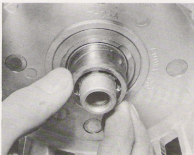
32.3e ... and the inner bush fitted
