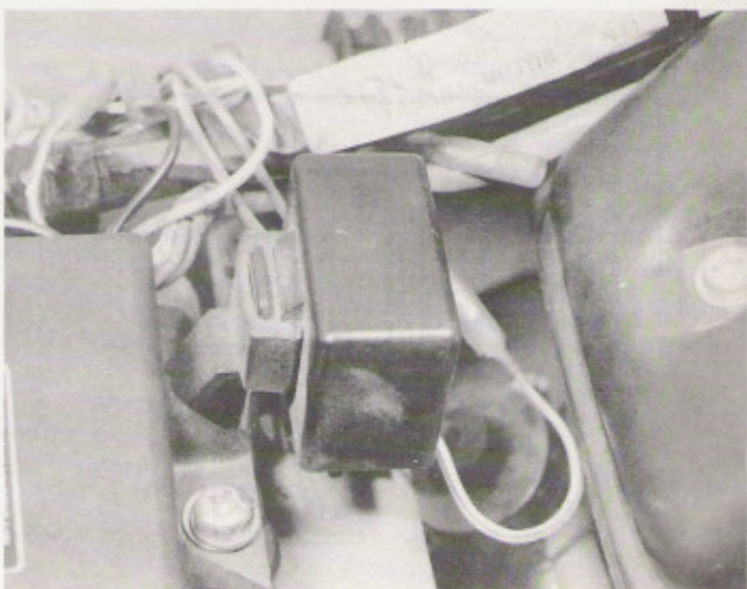
15.2 Rubber-mounted turn signal relay is fitted forward of the air filter casing
