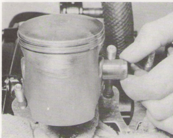
6.7b Gudgeon pins can now be displaced to allow the pistons to be lifted away
