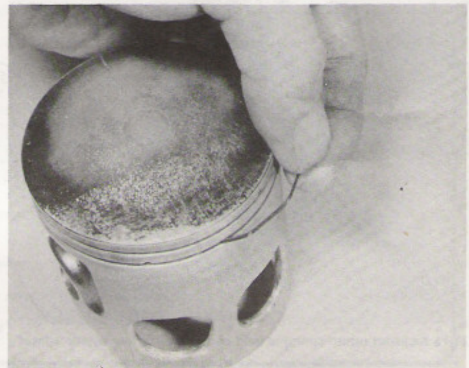
18.5b Scraper ring is backed by a thin steel expander
