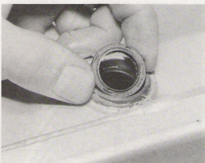
13.7a Fit new grease seals as required ...
