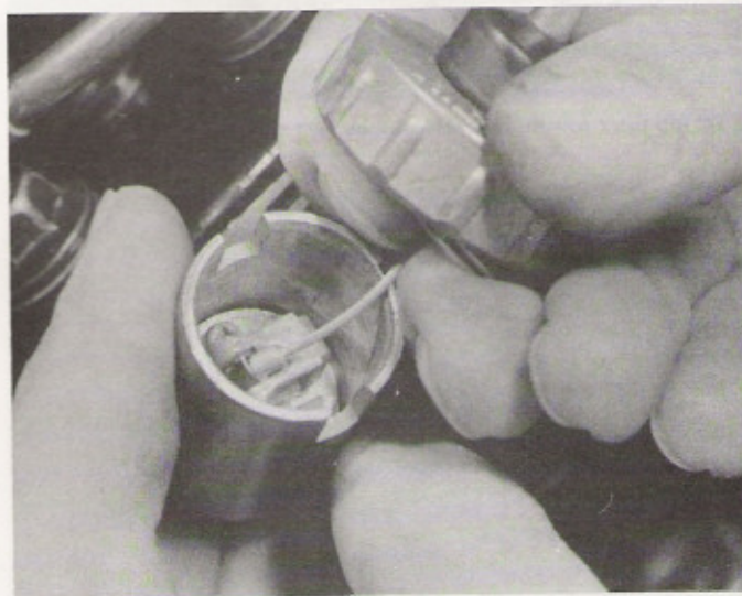
5.4 Compress the return spring, then disengage the inner cable
