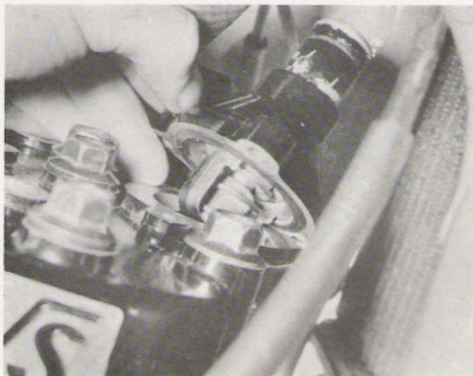
4.5d The thermostat housing and unit can also be removed to give improved clearance
