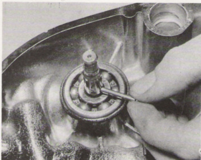
7.2c The driving pin must be displaced and removed to allow the shaft to pass through the bearing
