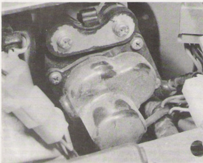
8.2a The YPVS servomotor is located to the rear of the steering head
