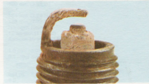
A worn spark plug not only wastes fuel but also overloads the whole ignition system because the increased gap requires higher voltage to initiate the spark. This condition can also affect air pollution
