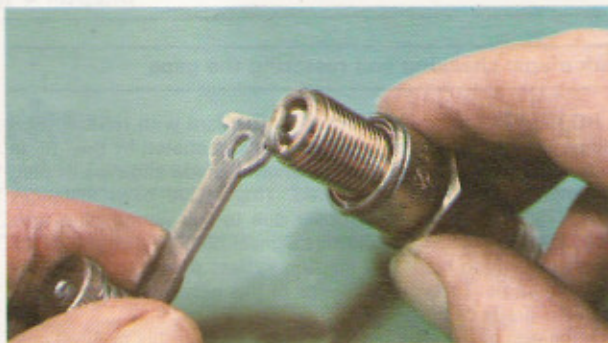
Altering the plug gap. Note use of correct tool
