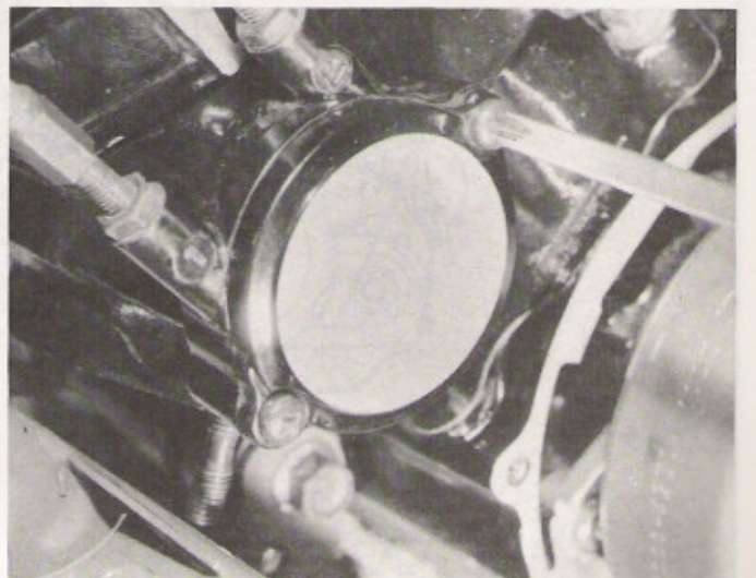
35.10e When correctly adjusted, refit the outer cover
