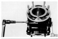
Lock the pulley with a spanner and remove the bolt connecting valves 1 and 2.
