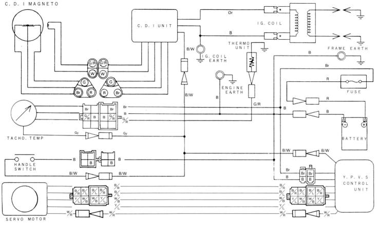
The wire harness designed specially for the TZR250 racer can be used with standard parts (excluding the ignition system).
