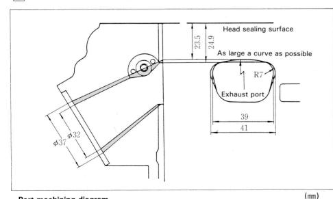
Port machining diagram
