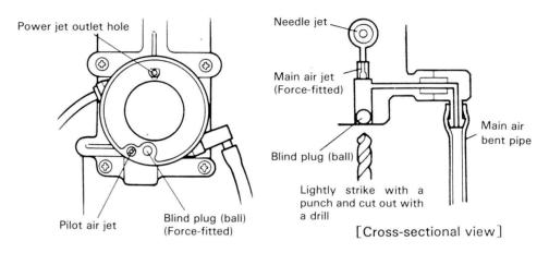
② The main jet is fitted in the body. Make a 2.5mm dia. through hole in the main jet (first start with making a 1.5 mm dia. hole air section only should be drill dimeter in steps). (The main air section only should be drilled.) Next, as shown, plug the air vent pipe hanging down from the carburetor.
