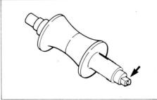
Use care not to scratch valve 1 (for the left cylinder) by gripping the pulley with pliers.
