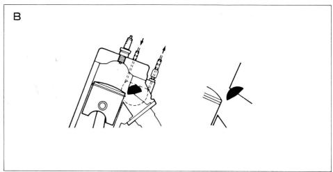
If it stops in the position shown in Fig. B, adjust it in the position shown in Fig. A by turning the adjuster.
