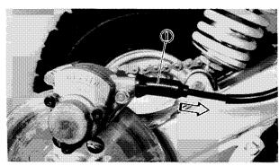
10. Pull back the cable adjuster cover ① from the rear brake caliper.
