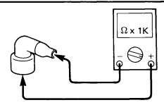
Check the spark plug cap for specified resistance.
