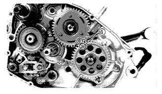
NOTE: \_\_ Note that there is the punched mark (1) on the drive gear and punched mark ① on the balancer
