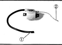
Check the secondary coil for specificated resistance.
