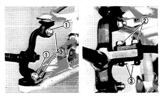
3. Inject grease from the nipples **6** using a grease gun until slight overflow is observed from the thrust covers.
