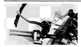
9. Loosen the locknut ① (Parking brake) and turn the adjuster ② clockwise to release the tension in the brake cable.
