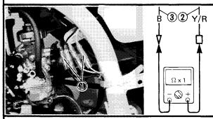
Check the lighting coil for specificated resistance.
