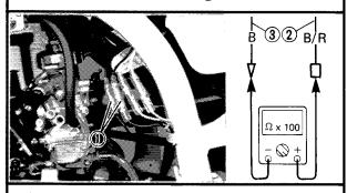
• Check the source coil for specificated resistance.
