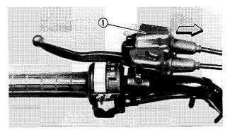
8. Pull back the cable adjuster cover ① from the clutch lever holder.
