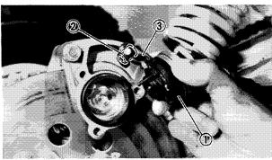
14. Take the adjuster unit ① out of the caliper body, and then detouch the pin ② from the adjuster arm ③.
