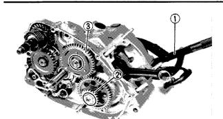
•Hold the rotor (CDI magneto) by the Rotor Holder ① to loosen the nuts (Primary drive gear ② and balancer gear ③).
