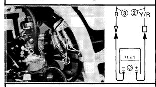
Check the lighting coil for specificated resistance.
