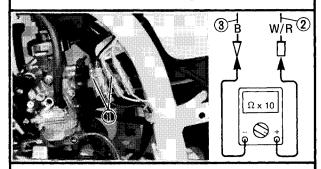
• Check the pickup coil for specificated resistance.
