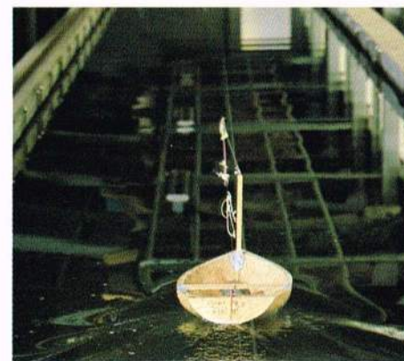
Hull models are tested in tanks to help find the best possible designs.
