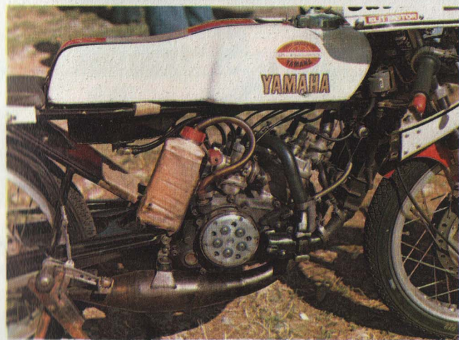
Under the plumbing live two tiny 60cc cylinders. The large canister is the oil-trap bottle for the breather system.
