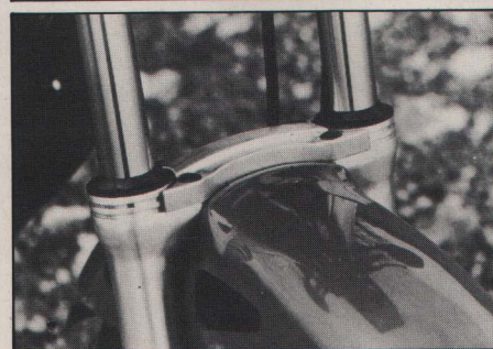
Top: Subtle adjustments to the fork of the FT500 make it handle more like a roadster than the dirt bike it was bred from. Top left: The four valve motor breathes through this monster CV carb. Middle right: Changes for road use include a deeper sump and electric starting. Above: The long fork legs benefit from the use of this fork brace and the steering's more precise for it. Right: Neat eh? Racer type rear spindle adjusters.
