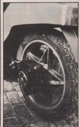
The Phasar is built to take a choice of three engines, CX500, BMW or Z1300, all with shaft drive.
