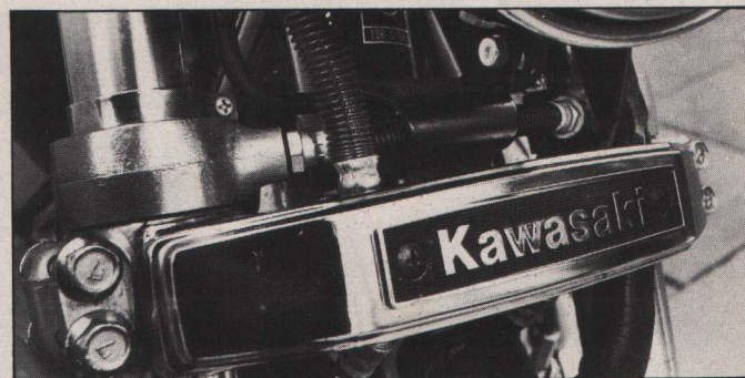
All the linkages are dealt with neatly, the hose running across under the headlight balances the air fork.
