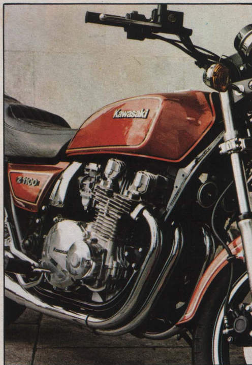
Big fuel tank is deceptive. Nominal capacity is over 4½ gallons but the most we could squeeze into it was four.
