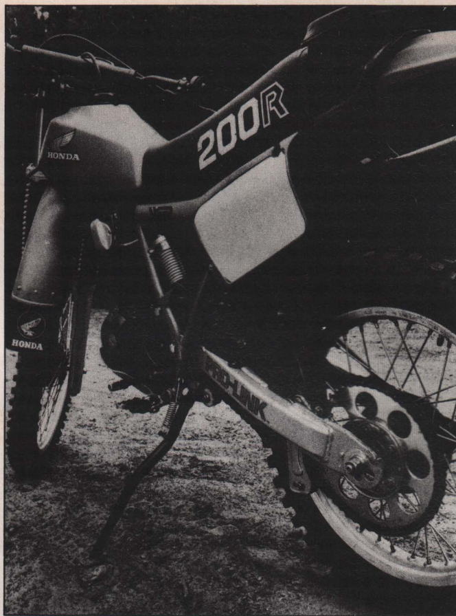
The serious end of the new XR200R: the Pro-Link allows it to reach parts the old model couldn't.
