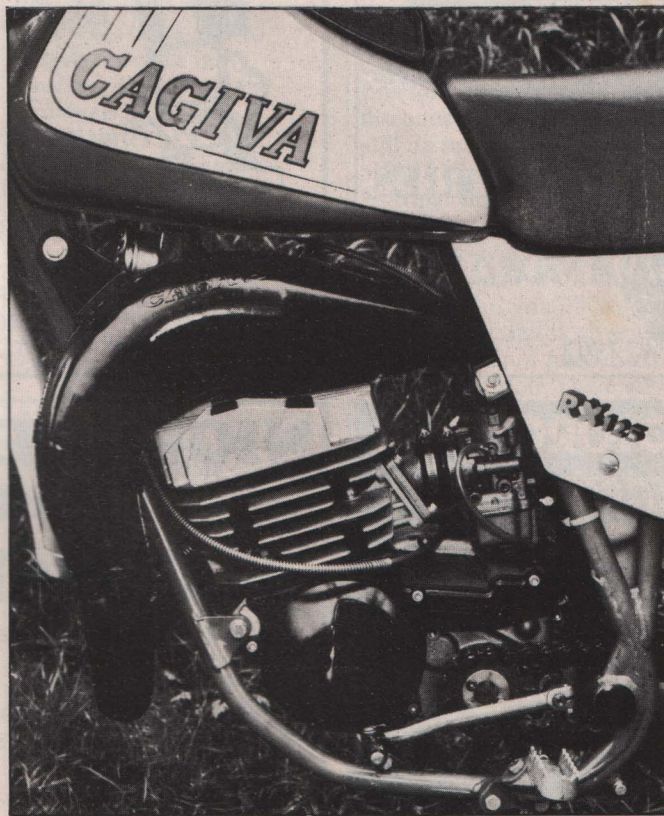
Modest expansion chamber gives an indication of tractability; stepped ignition cover keeps gear lever tucked in.
