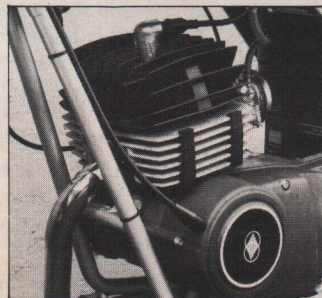
Gilera's semi-double cradle frame.
