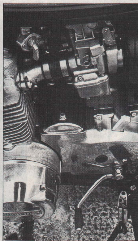
These Dellorto carbs have a progressive choke. Gear lever works better than it looks.
