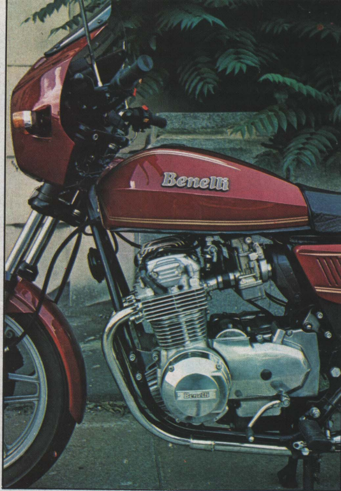
Benelli's single overhead camshaft 604cc four is an example of Japanese-inspired design and Italian flair – an odd combination.
