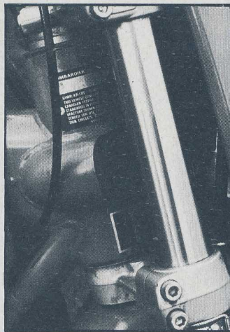
Air filter intake on the Can-Am is on the headstock.
