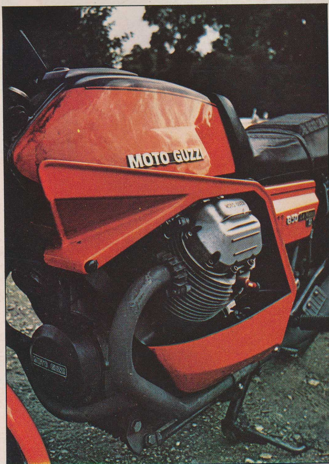
Left: The design of the fairing allows good cooling for the pots and some warm air through to the legs. Above: Black exhaust and rear shock springs contribute to the Guzzi's understated look.
