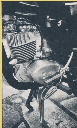
Engine of the TS150 is based on the same motor as the BSA Bantam.
