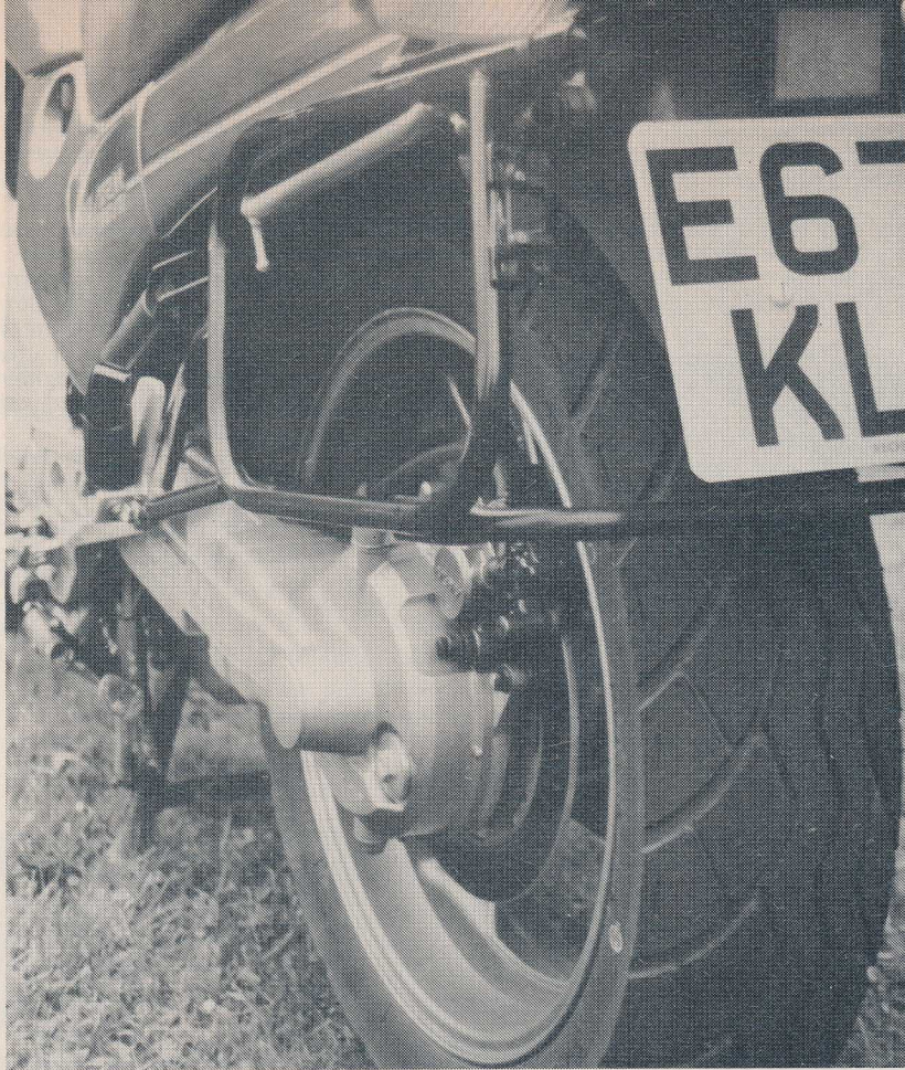
Rear disc inboard of the shaft drive on the single 'Pro Am'. Wide radial tyres on 17 inch wheels enhance handling.
