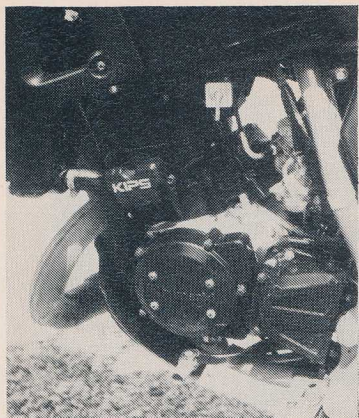
'KIPS' is Kawasaki's power valve system which monitors exhaust resonance and boosts power through the rev range.
