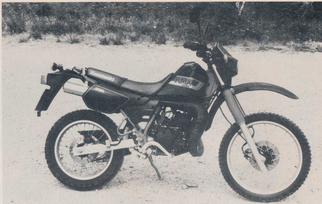
'KIPS' is Kawasaki's power valve system which monitors exhaust resonance and boosts power through the rev range.
