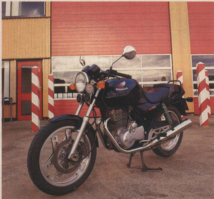
Four years on and the 'G' model has changed from the 'F' with a beefed up starter motor only.
