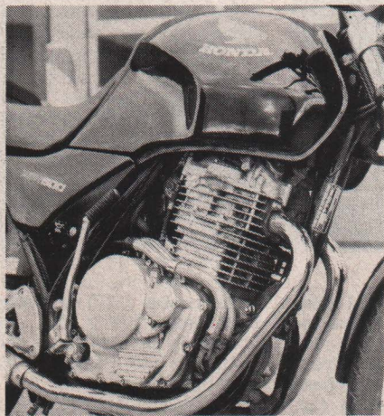
Engine specification is borrowed from Honda XR500 enduro bike but no parts are interchangeable.
