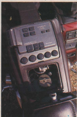
Fill up under the flap on the false petrol tank and strike up the band with the built-in stereo radio/cassette. ZZ Top or Chopin, sir?
