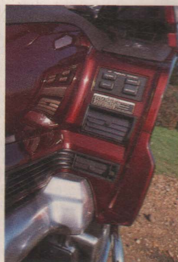
Controls on right of fairing for adjusting rear suspension.
