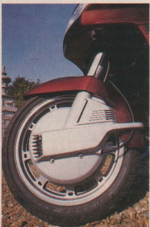
Twin front discs are fully enclosed and there's a single disc at the rear. Probably the Wing's poorest feature, the brakes could only be described as adequate.
