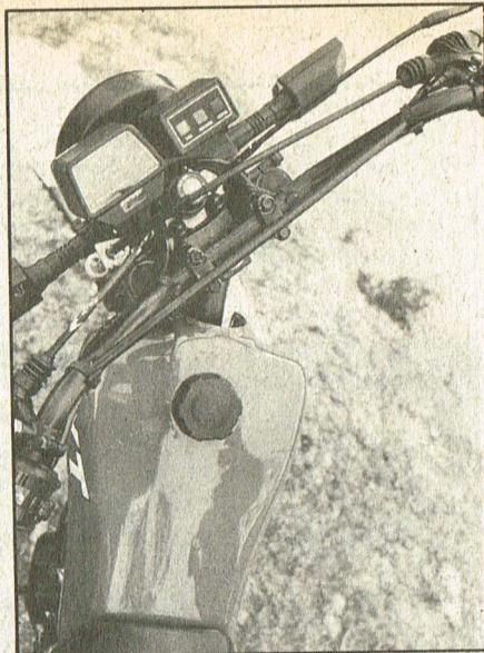
Street riders are catered for a little more with the idiot lights beside the XT's speedo (left), yet funnily enough the Yamaha's clocks are also better in the dirt than the Honda's, which is too vulnerable.
