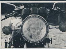
The bike's superb Koito H4 halogen headlight is one of the best standard units around and better than most Japanese QIs. The XS11 dual horns are good too. Instruments are steady and easily-read though binnacle could do with modernising. Bike does not have modern steering lock position.
