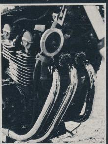
pletely out of character with its smoothness elsewhere in the rev range, ignoring the throbbing at idle and very low engine speeds. Unfortunately, these vibes occur at the most commonly used touring speeds in top gear (105 to 125 km/h'índicated) and are a pain in the neck when cruising at reasonably legal speeds. The engine cries out for rubber mountings like the XS1100 has, but until it gets them keep running a spanner over any bolts that might loosen every month or so.
