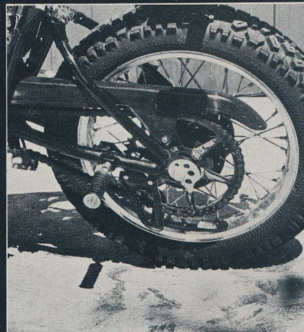
The 17-inch wheel of the Yamaha, shared with the Kawasaki, and just too small for adequate grip and traction.
