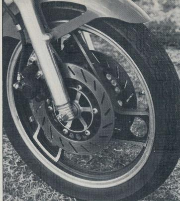
Front ends take a different tack. The RZ's enormously powerful twin discs win the stopping war from the VF's enclosed single unit, but the Honda's antidive-equipped forks are better in initial compliance.
