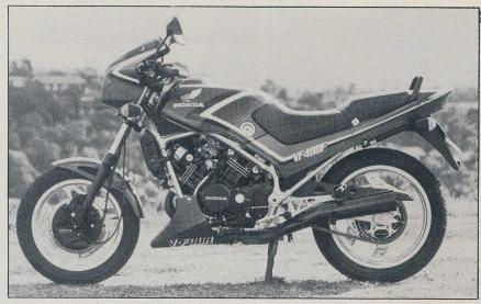
Water-cooled 90-degree V-four four-stroke, crankshaft set transversely. Double overhead camshaft driven by HyVo chain, four valves per cylinder. Barrels cast integrally with top of crankcase. One-piece crankshaft, plain main and big end bearings. Wet sump lubrication.
