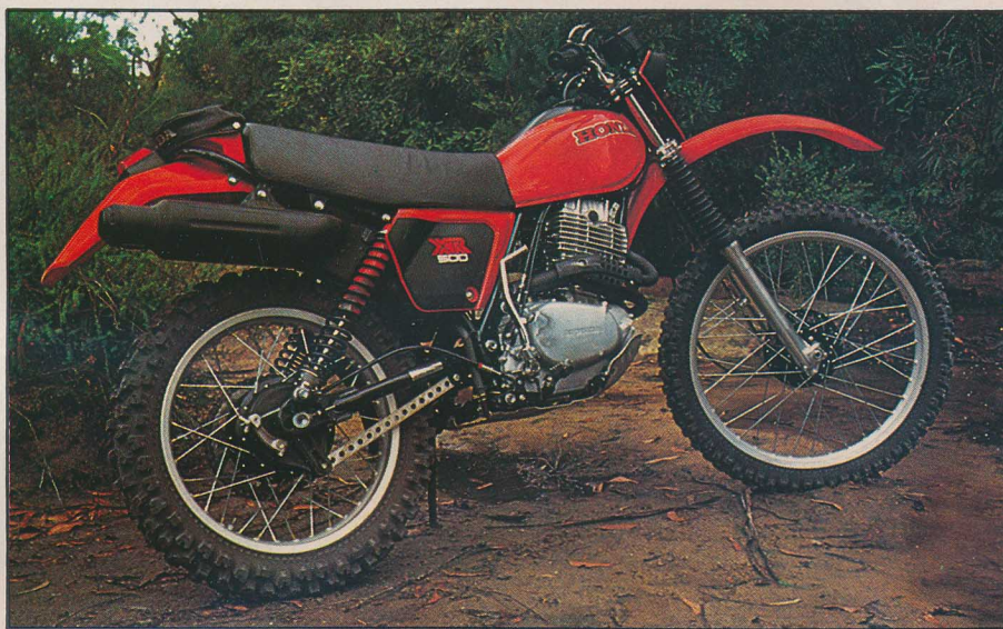
Honda's latest XL variant features the much-advertised 23 in. front wheel and many design features of the lighter XR500. Bike is nevertheless a BIG machine!
