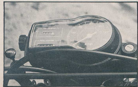
Revised XL instrumentation is a welcome relief from the speedo/tacho pack of older XL350s. Bar-mounted choke is convenient and the speedo/tripmeter is well-suited to the needs of the casual dirt rider.
