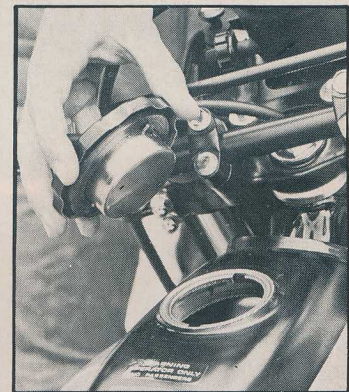
Both tanks use large, easy-fill cap and hold 10 litres.
