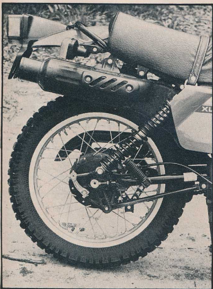
The bulk of the street. XL street/trail rear end (left) features bulkier muffler/spark arrestor, ADR legal lighting, flexi-mount blinkers and steel inner guard. Steel torque arm and less refined suspension are disappointing touches! The more refined XR rear end carries small, light toolpouch, plastic guard and still bulky muffler. Suspension performance outstrips that of both the XL and Yamaha's latest TT/XT models.
