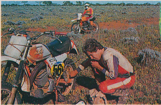
Apart from two flat tyres, a front end that's shot and no spark it's running fine. We're kidding. The first flat for Peter Carter was my chance to see how the horseshoe-shaped tubes work. First you have to cut the old tube to get it out of the swing arm, then hassle to get the special double-ended one in, then the tyre back on, all the time keeping the bike on the stand and not falling over in the sand. Then pump the tyre up and wait a minute to find you have pinched it, or the end has blown out, or the initial puncture was not a pinch but a sharp stick or thorn and it's still in there. I think the U-tube idea is useless. I gave Peter one of my tubes.
