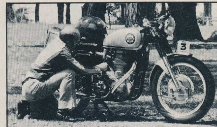
Finally, when all else fails, it's necessary to strip half the magneto in the fond hope that a cure can be found. In this case, the magneto had coughed its last and the bike had to be taken back in a trailer.
