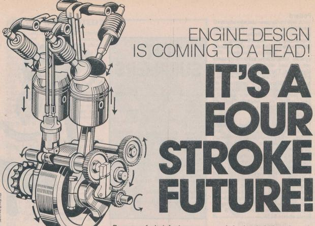
The ultimate big-banger four-stroke twin? Not yet it's not but the Norton-Cosworth is still ripe with promise thanks to advanced detail design including eight-valve head and water cooling. Engine's an integrated part of the bike's frame.
