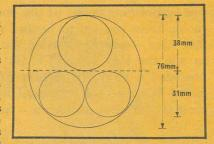
Figure 1 shows how two smaller values fit into the same space as one larger valve and combine to give more port area. A 38 mm circle takes half a 76 mm bore, for example, and has 1134 mm<sup>2</sup> area. But the same size semi-circle also takes two 31 mm circles which have 1509 mm² area combined. Fourvalve chambers also give good central spark plug location.
