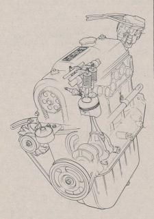
Honda's CVCC design, the first stratified-charge engine in production, is used in Civic car to meet anti-pollution laws in USA and Japan. Unique head has three valves and two chambers a cylinder. Normal inlet valve supplies very weak air-fuel mixture to cylinder. Tiny auxiliary valve feeds richer mixture to ignition chamber where it's fired by the sparkplug and, in turn, lights the main charge.
